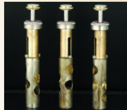
Notice the wear and corrosion on Trumpet X's pistons. Especially the large amount on #2 and #3. Also note the yellow discoloration of the pistons. This is brass that has been deposited on the pistons from the valve casings. At this point all three pistons were ruined and no longer functioned.
